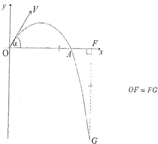
In the diagram above, a projectile is fired from a point O at the top of a vertical cliff. Its initial speed is  $V \text{ m/s}$  and its angle of elevation is  $\alpha$ . Let the acceleration due to gravity be  $g \text{ m/s}^2$ .
